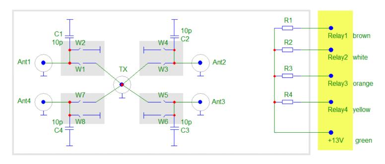
W1-W2 = SPDT W2, W4, W6, W8 on when relays off
